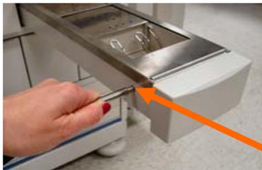
The single-item access drawer belt can be manually moved by using the slotted key to rotate the pin.
